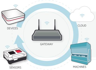
Fog computing not only uses an on-premise gateway to manage the process of communication between sensors and actuators to the cloud, but it introduces a degree of local, cloud-delegated, control. Software running on a local gateway has responsibility for managing the flow of data to and from edge nodes, provides an element of local autonomous control in addition to building in the capability to communicate with legacy and modern devices.
